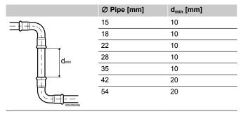
Two pressfittings too close together can compromise the seal of the joints. Note the minimum distances.
