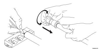
Press the fitting onto the pipe with the appropriate tool and visually check the result.
