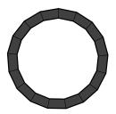
If the fitting is not pressed, the particular profile of the o-ring identifies the irregular condition, both during the seal test and visually/audibly, through leaking of water or air. This characteristic is commonly known as "unpress - untight". After the fitting has been pressed, the o-ring easily closes all the flows, ensuring the hermetic seal as with the traditional type.
